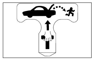
There is a glow-in-the-dark trunk release handle located on the latch inside the trunk. This handle will glow following exposure to light. Pull the release handle to open the trunk from the inside.
